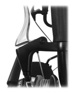
4) The platform is set in the forward position. In can be angled inward, by taking out the two rotational bolts on the stem, and rotating it inward to either the 30, 60 or 85 degree position. Reinstall bolts once desired position is selected.
