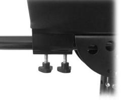
3) The distance of the reach of the brake handle can be adjusted smaller by tightening the set screw on the front of the brake handle. By making this adjustment, it might require a minor cable adjustment.
