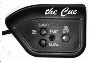
period from 4 to 28 minutes in increments of 4 minutes; each click that sounds after pressing the button indicates 4 minutes of operating time in effect (from 1 to 7 clicks). Pressing the lower button lowers the click volume in steps to the softest setting, then recycling to the loudest setting.
