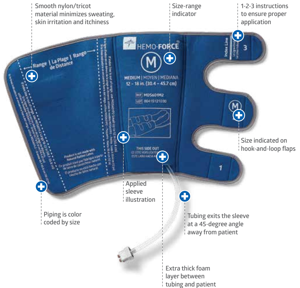
Hemo-Force II intermittent sleeves features a pull-apart tube connector for quick disconnection
