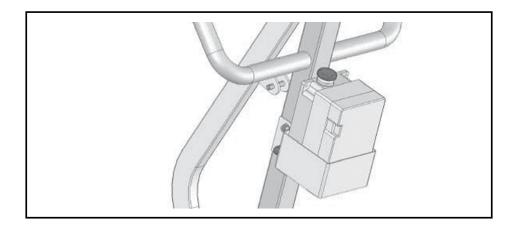
6. Place the control box in the bracket, as shown above.
