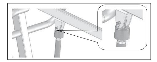
8. Attach the actuator top to the boom bracket and insert retainer pin, as shown above. Insert retaining ring through retainer pin hole to secure actuator top to boom bracket.
