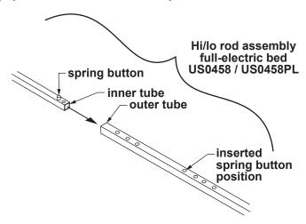
Depress spring button and insert inner tube into outer tube until first hole of second hole set is reached as shown above. Release spring button to lock it into hole.
