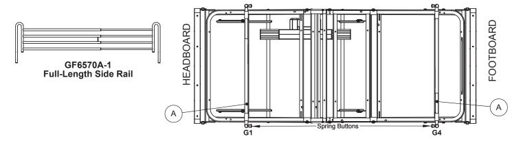
Position spring-loaded crossbraces #A into slots G1 and G4 on both sides of bed with spring buttons facing inward as shown above.
