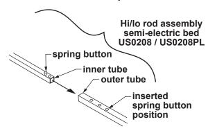
Depress spring button and insert inner tube into outer tube until third hole is reached as shown above. Release spring button to lock it into hole.
