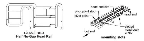
The Half No-Gap Head Rail, shown above, provides full head coverage of 31.5 inches and extends to eliminate the gap between the head board and the end of the rail. The GF6590BH-1 mounted on the bed's head and the GF6580BH-1 mounted on the bed's foot combine to create the Patriot split rail system.
