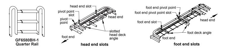
The Quarter Rail, shown above, is approximately 18 inches in length when mounted on the Patriot bed. It can be used as a head assist, head rail, or foot rail.
