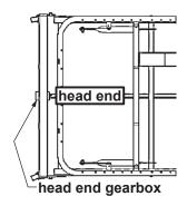
Fig 3: All Bed Models: Attach hi/lo rod assembly to head end gearbox
