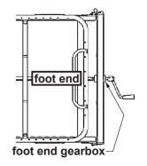
Fig 1: Semi-Electric Bed: Attach hi/lo rod assembly to foot end gearbox
