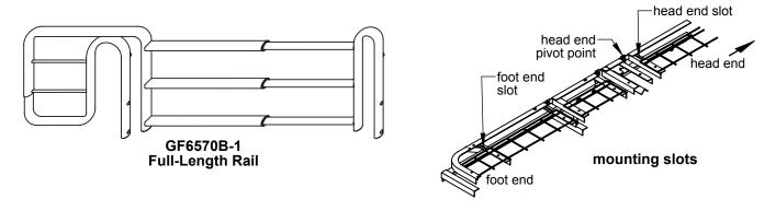
The Full Length rail, shown above, is a nominal, telescoping full length rail that provides maximum length rail perimeter coverage.
